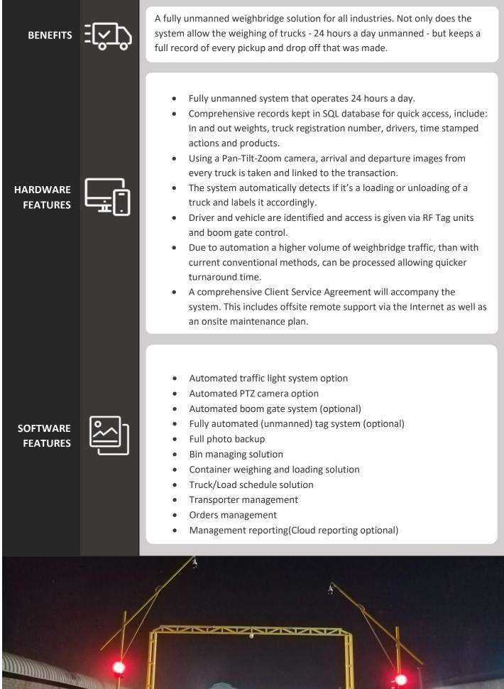
Unmanned weighbridge system is activated by means of a predefined, coded, inexpensive RF tag. Each driver will receive is own unique tag which is registered to himself or the vehicle.
